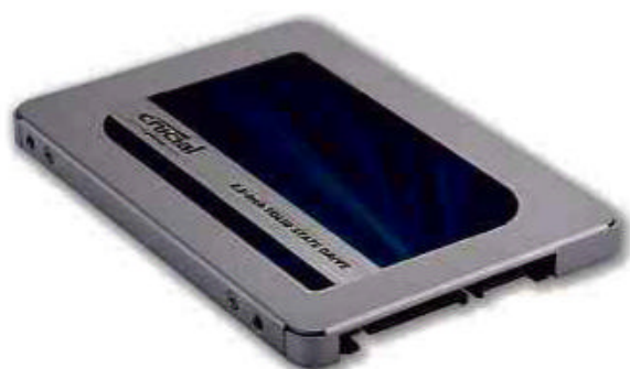
2.5in SATA SSDs can replace the traditional 2.5in hard drives found in most laptops
