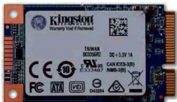
mSATA use the same SATA interface as 2.5in SSDs, but takes up less room
